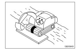
When operating in water or when crossing shallow, check the bed soil condition and depth and flow speed of water, then proceed taking care that water is not above carrier roller.
