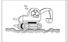
When working on soft ground, place mats or wood boards on the ground to prevent the machine sinking.
